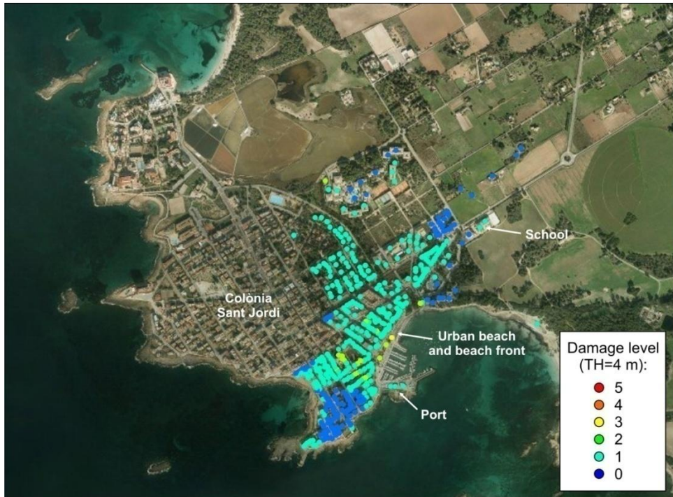
Figure 3.3.19. Damage level calculated for a limited area within Colònia Sant Jordi test site and a tsunami height of 4 m.
