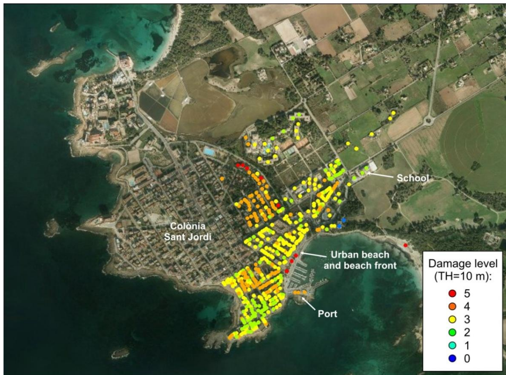
Figure 3.3.21. Damage level calculated for a limited area within Colònia Sant Jordi test site and a tsunami height of 10 m.
