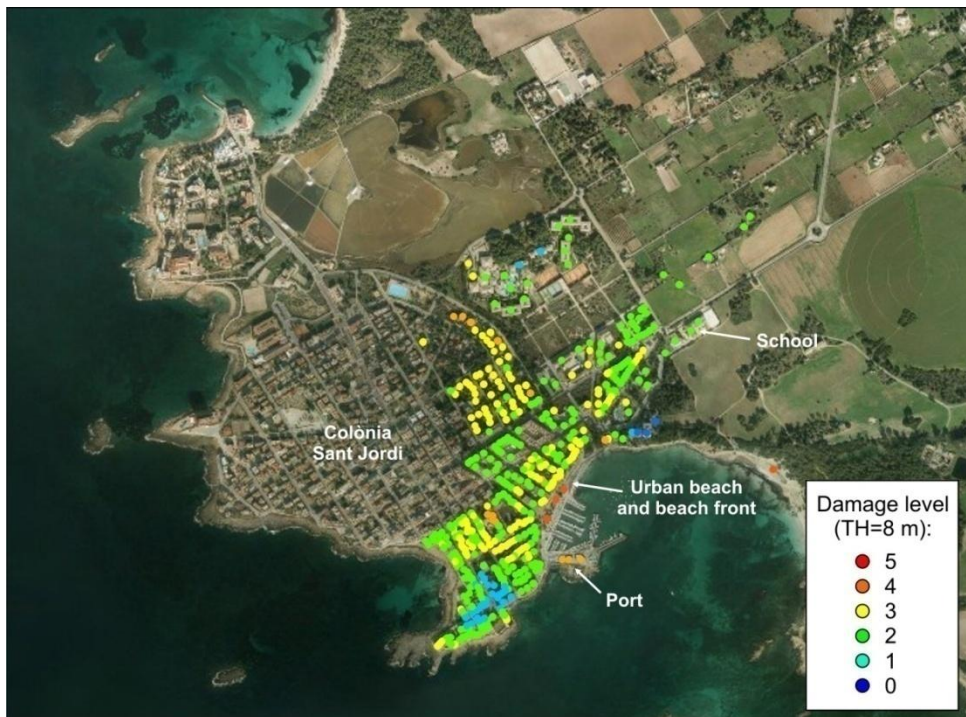
Figure 3.3.20. Damage level calculated for a limited area within Colònia Sant Jordi test site and a tsunami height of 8 m.
